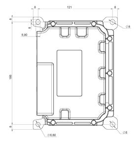
Top material: plastic injection molded, bottom: metal sheet
